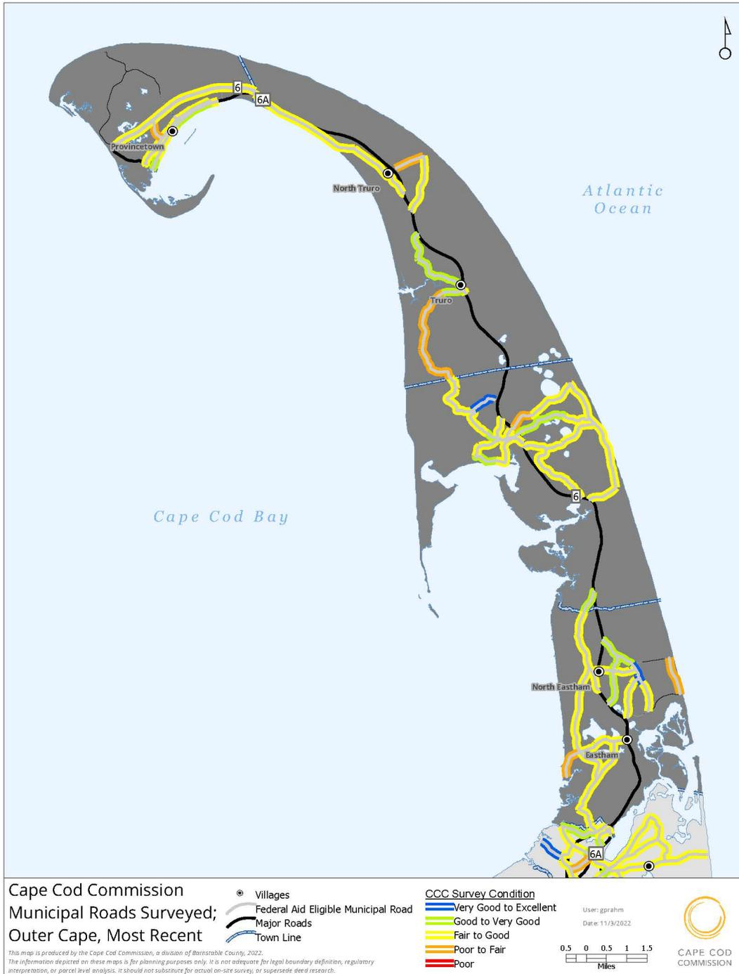
FIGURE 7. Pavement Condition Surveys: Outer Cape
