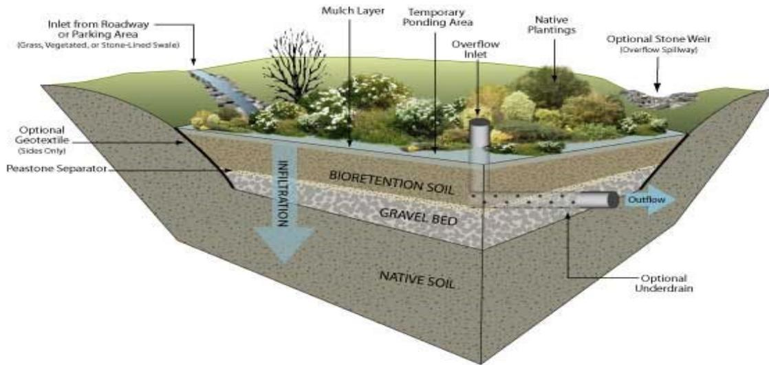
FIGURE 15. Bioretention
