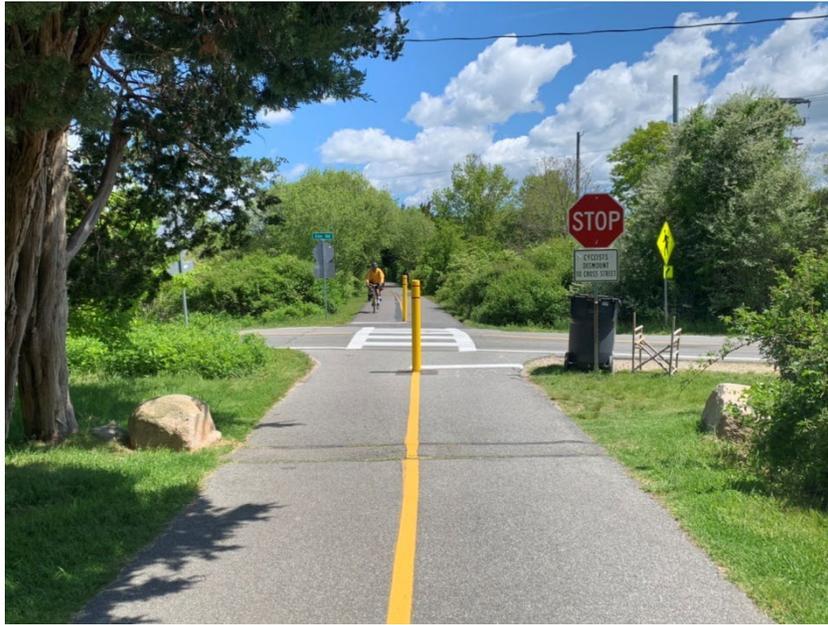
*Figure 24: Advance Warning Signage with Faded Pavement Markings*
