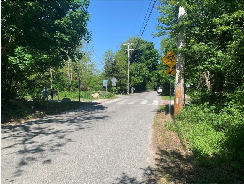
*Figure 45: A Wide Crosswalk and Ladder Markings Improve Intersection Visibility*
