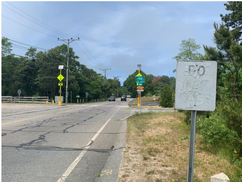
Figure 177: Trail Crossing is STOP Controlled. Facing SB, There is Only a Single RRFB.
