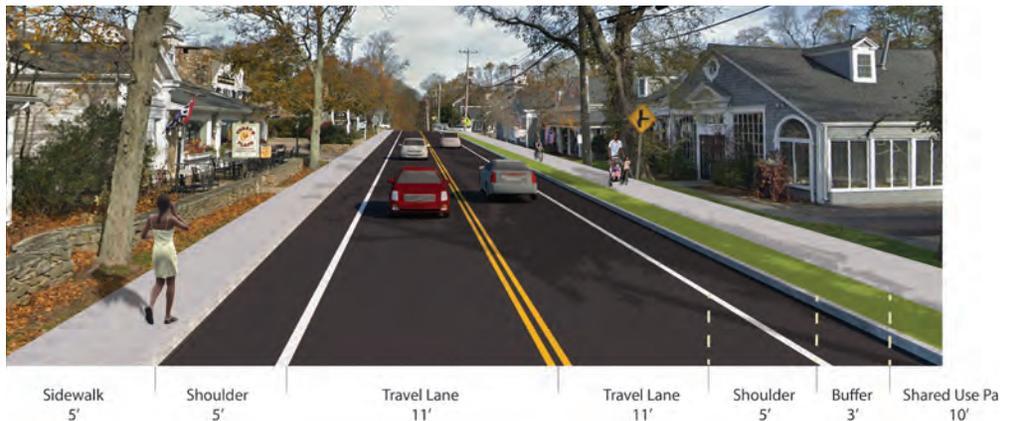
Figure 28. Town Mix Cross Section Ranges with Onstreet Bike Lanes
