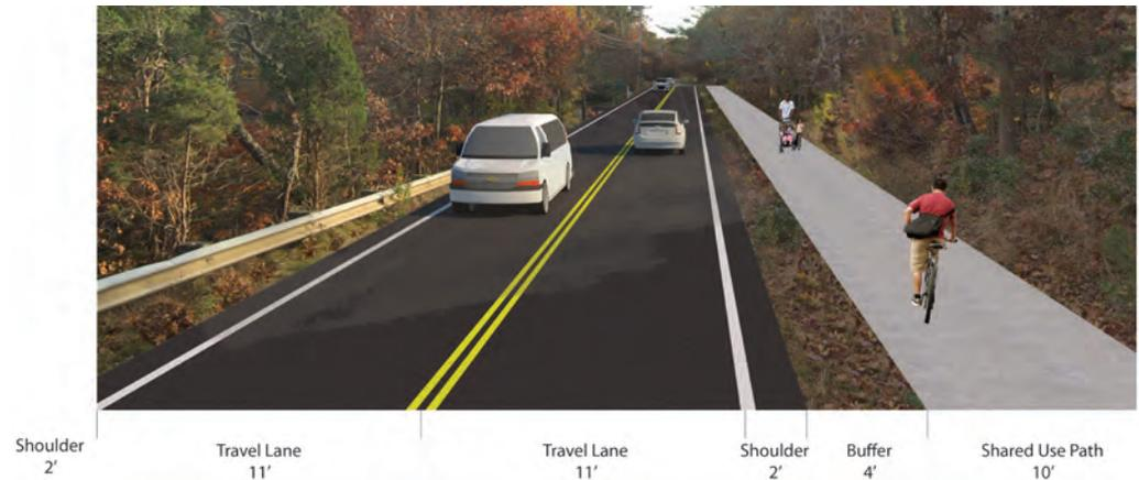
Figure 37. Rural Residential Cross Section Ranges with Shared Use Path
