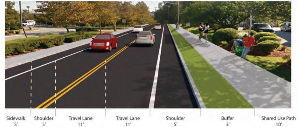
Figure 32. Suburban Commercial Center Concept with Onstreet Bike Lane
