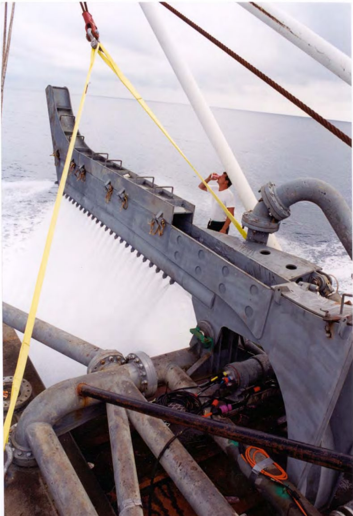
Photograph 3: Water nozzles on plow stinger
