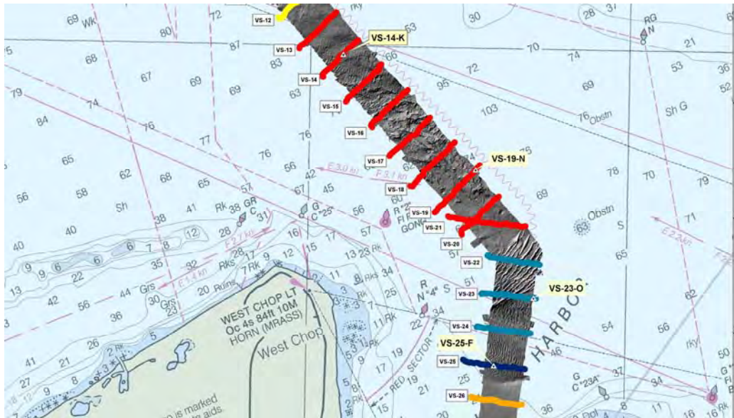
Red transects of Gravel Pavement (boulders) in deeper water of the southern half of the Eversource 5 th Cable Corridor
