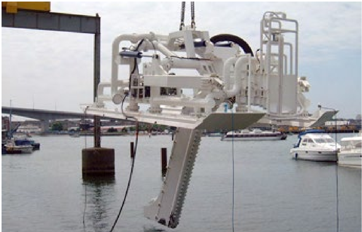
Photograph 2: Hydroplow showing burial stinger extended
