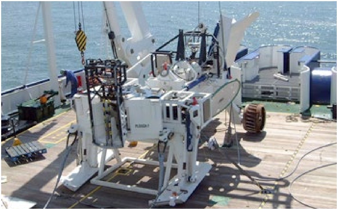
Photograph 1: Typical hydroplow on deck
