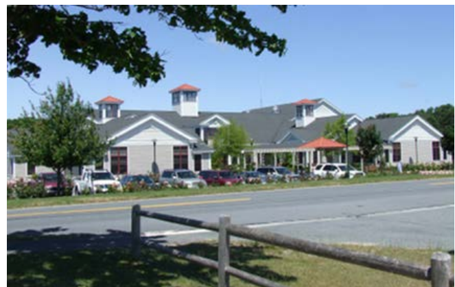
Figure 7 The Harwich Community Center incorporates varied roof heights and forms to break down the overall scale of the building.
