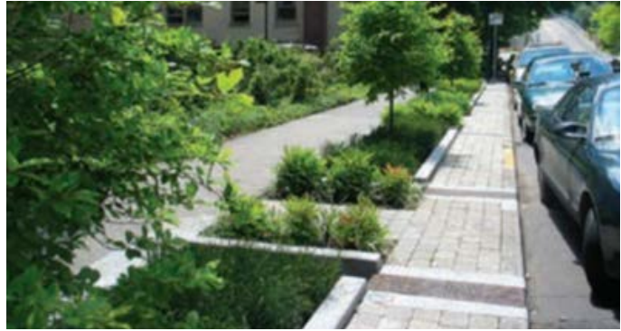
Figure 28 Layers of plantings through pedestrian areas also serve as stormwater management areas. (Vermont Urban and Community Forestry Program, 2018)
