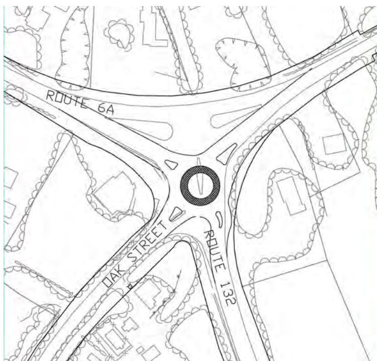
FIGURE 4 - ROUNDABOUT CONCEPT: RT 6A, RT 132, OAK ST IN BARNSTABLE
