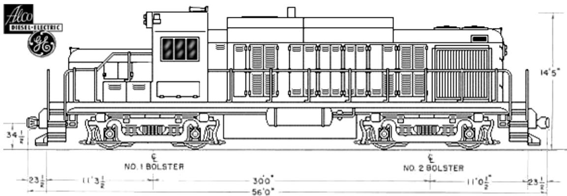
FIGURE 36: DIAGRAM FOR ENGINE 1201
