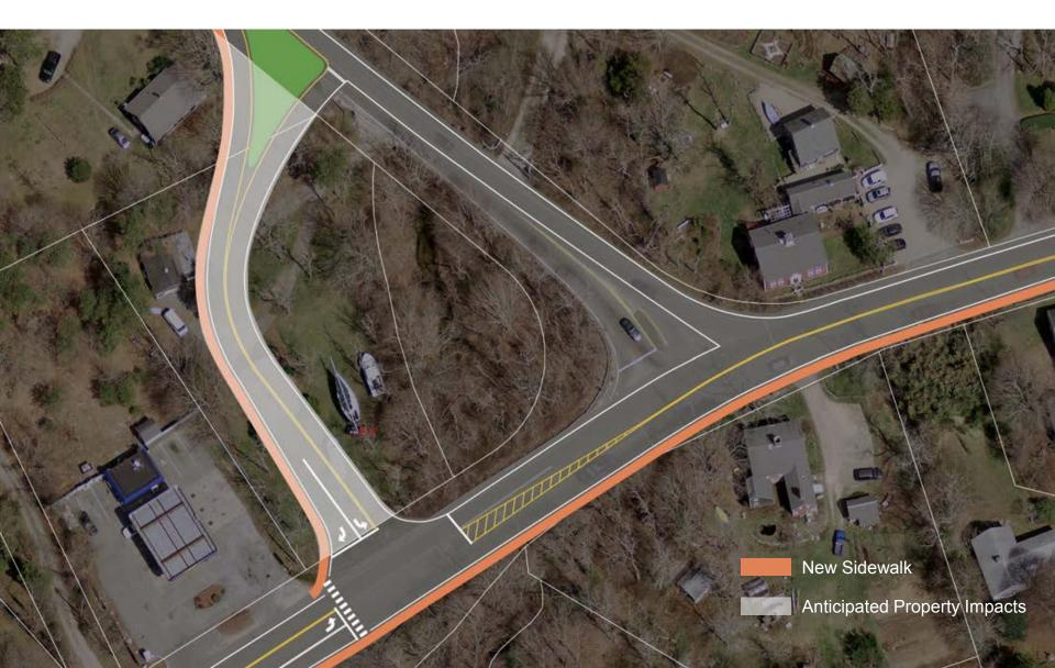
Relocate/realign intersection to the west
