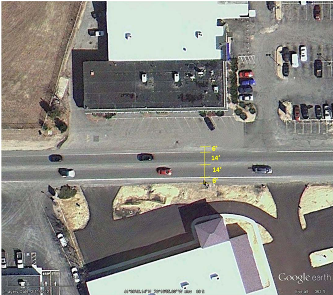
FIGURE 12 - RT 28 PAVEMENT WIDTH (EAST OF AUTOZONE)
