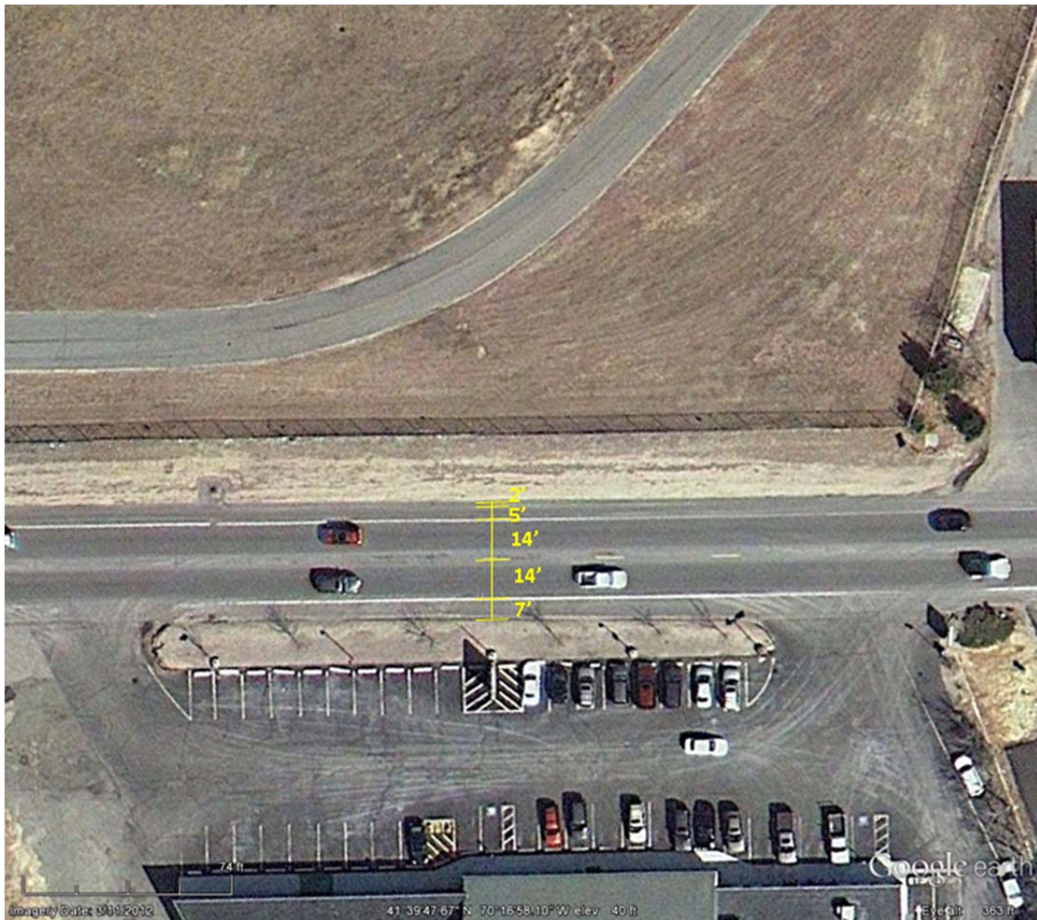
FIGURE 11 - RT 28 PAVEMENT WIDTH (WEST OF AUTOZONE)
