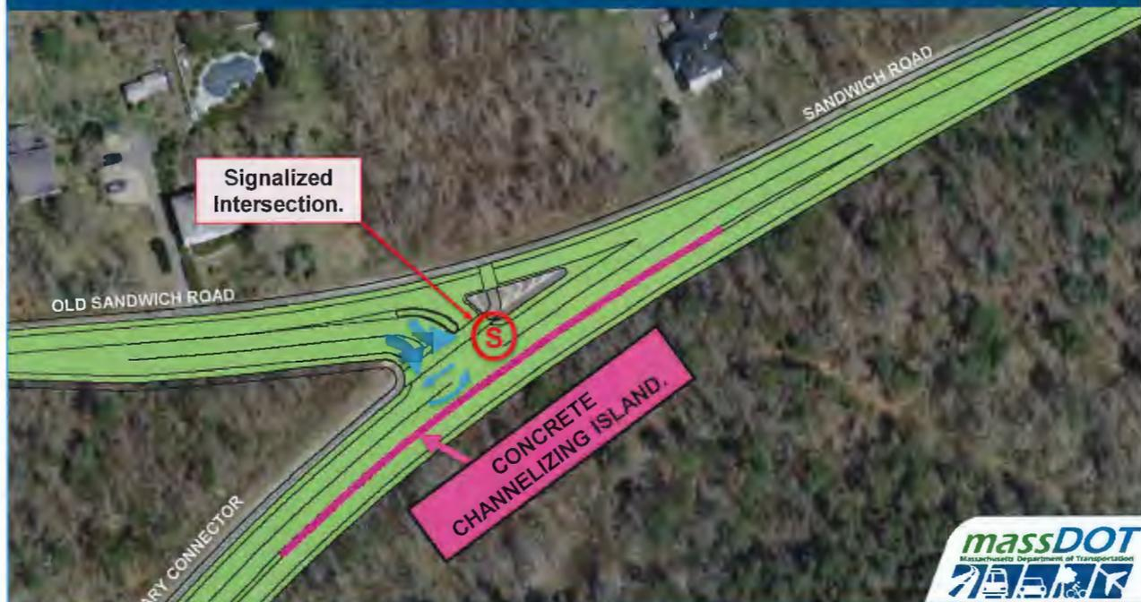
Proposed: Signalized Intersection. Includes through-lane from Bourne Rotary Connector to Sandwich Road and ADA-compliant sidewalks and crosswalks.
