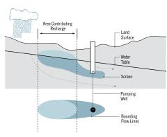
Diagram WR2: Wellhead Protection Recharge Area
