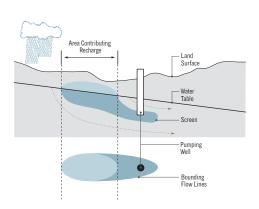
Diagram WR2: Wellhead Protection Recharge Area
