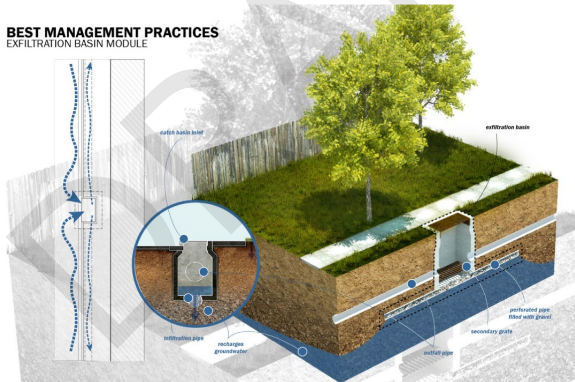
FIGURE 12. Leaching Catch Basin
