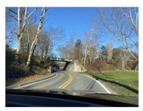
Image 1: Dashboard view of a low clearance bridge across Route 6A. In this location, heavy vehicles often collide with, attempt to reverse, or turn around from the bridge.
