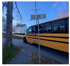
Image 4: School bus turning left from Route 6A on to Old Jail Lane. The approach only wide enough to accommodate one vehicle despite being a two-way road.
