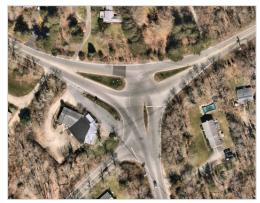
Image 5: Aerial image of existing conditions of Route 6A at Route 132 and Oak Street, showing large footprint of intersection and wide approaches.
