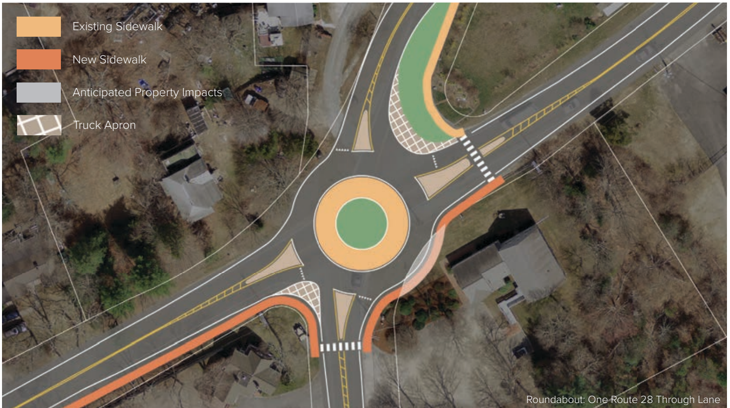
Roundabout: One Route 28 Through Lane
