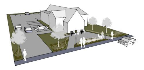
FIGURE 16: MOVING PARKING TO THE SIDE AN REAR ALLOWS THE FRONT SETBACK AREA TO BE USED FOR PEDESTRIAN AMENITIES AND TO ENCOURAGE ACTIVITY ON THE STREET. LANDSCAPING, HARDSCAPE AND STREET FURNITURE CAN BE INCORPORATED TO IMPROVE THE APPREARANCE OF THESE AREAS AND REDUCE THE AMOUNT OF VISIBLE PARKING AND PAVEMENT.
