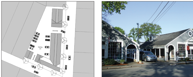
Figure A34: The shared parking for this Falmouth commercial site is located to the rear of the property and behind the street fronting buildings (diagram above left); the parking is accessed via narrow driveways between buildings that shield the parking from view.
