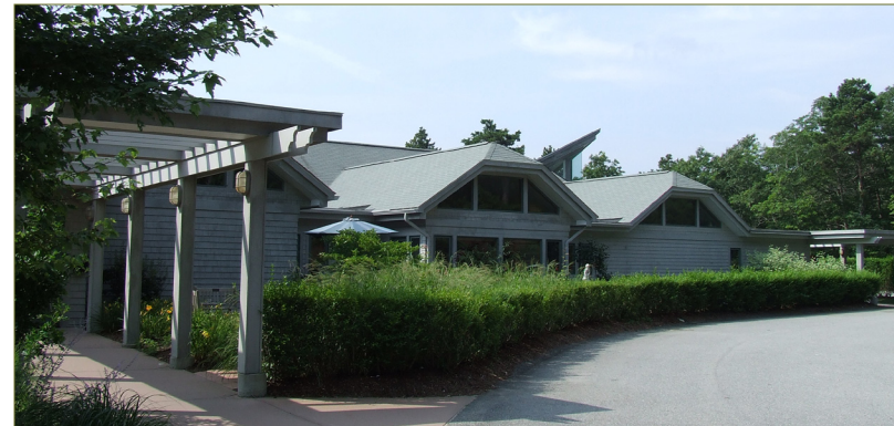
Figure B20: This building in Sandwich uses a pergola, varied eave lines, and multiple ridge heights to give the building a pedestrian scale.
