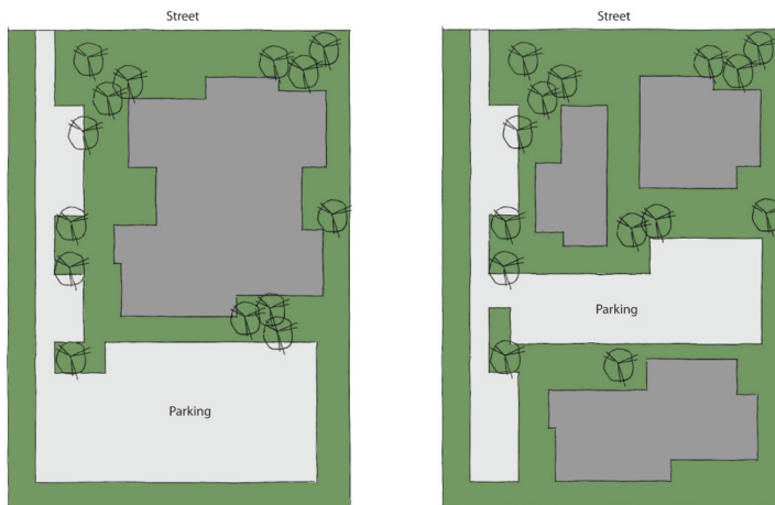
Figure B1: Rather than constructing a single, large building mass (left), consider breaking the building area into several small building masses clustered around a focal point (right).
