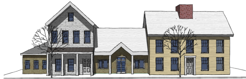
Figure A6: Variation in height, orientation, and setbacks create interest and continue the rhythm of facades along the streetscape, as illustrated in this sketch.
