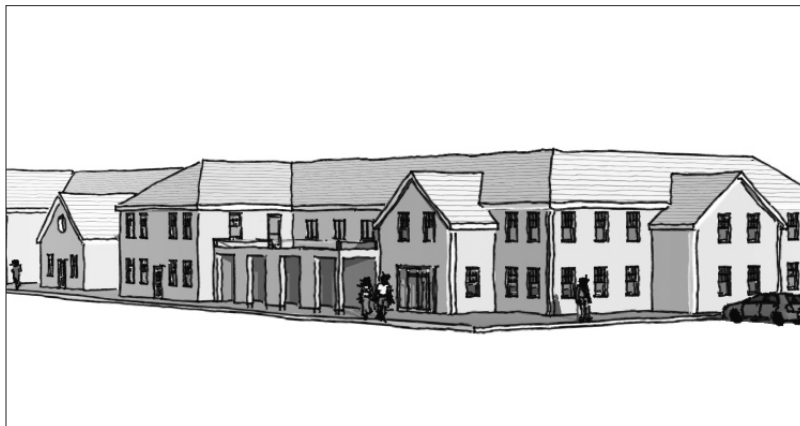
Figure B18: As shown in this sketch, lower roof heights on attached masses reduce the apparent scale of the building.
